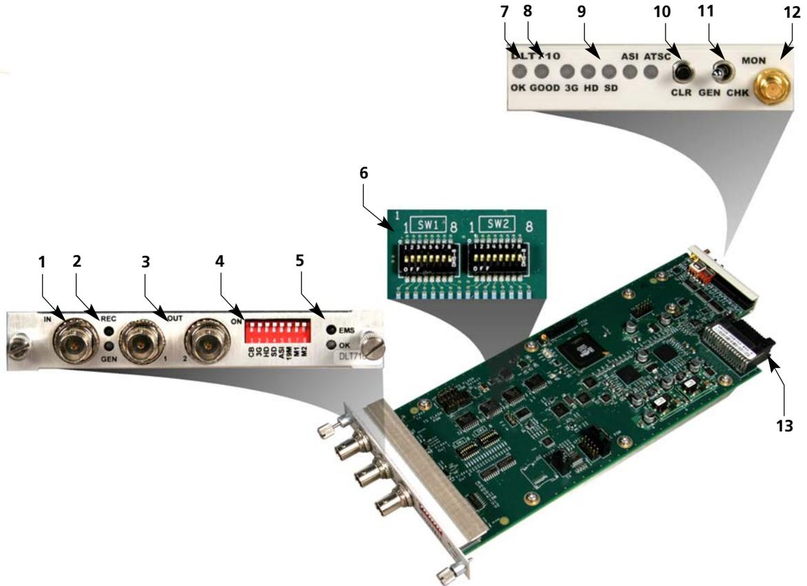
**Figure 13. DLT710 Module Major Components**
