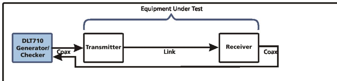
**Figure 1. End-to-End Check Using One DLT710**
