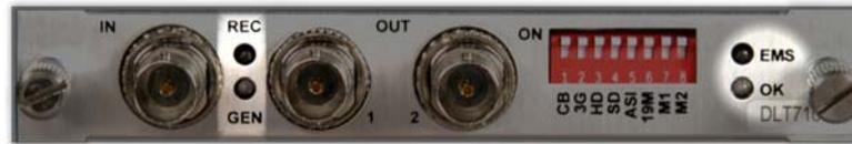
**Figure 20. DLT710 Rear Panel Status LEDs**
