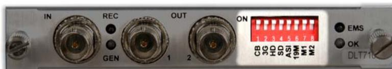
**Figure 16. DLT710 Rear Panel Configuration DIP Switch**
