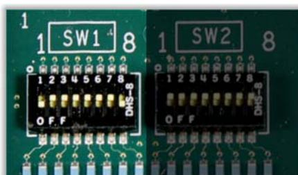
**Figure 14. DLT710 SW1 Configuration DIP Switch**
