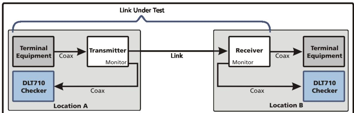
**Figure 4. DLT710 Monitoring Two Live Links Using Coax**
