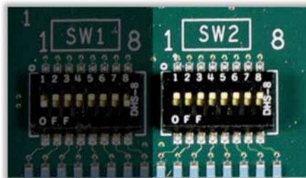
**Figure 15. DLT710 SW2 Configuration DIP Switch**
