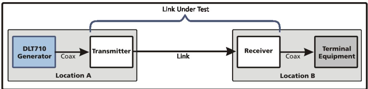
**Figure 3. DLT710 Test Video Delivered To Terminal Equipment**
