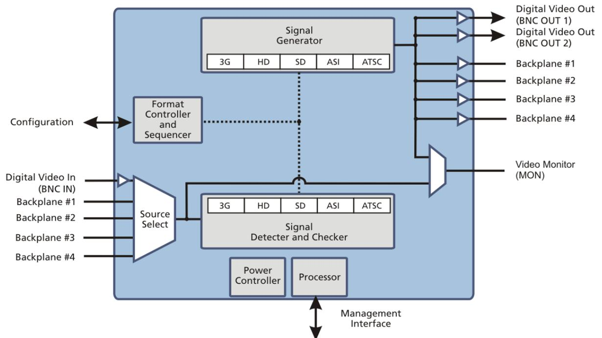
**Figure 12. DLT710 Module Functional Block Diagram**
