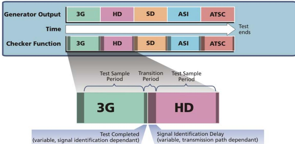
**Figure 10. Multi-Format, Single Pass Mode**
