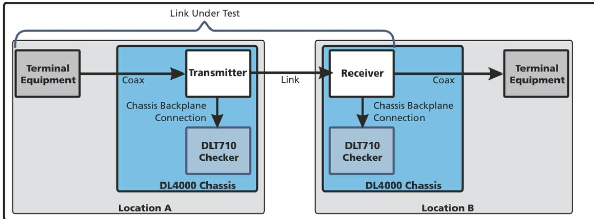
**Figure 5. DLT710 Monitoring Two Live Links Using Host Chassis Backplane Connections**
