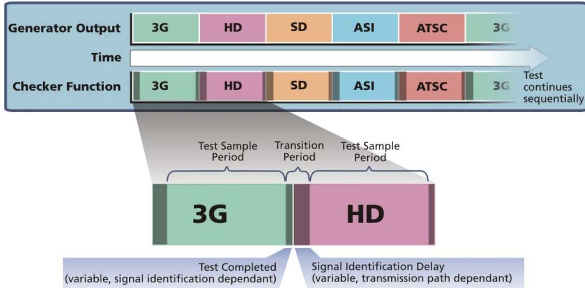
**Figure 11. Multi-Format, Continuous Mode**
