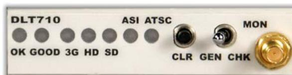
**Figure 19.** DLT710 Front Panel Status LEDs and Monitor Connector
