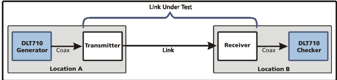
**Figure 2. End-to-End Check Using Two DLT710 Modules**
