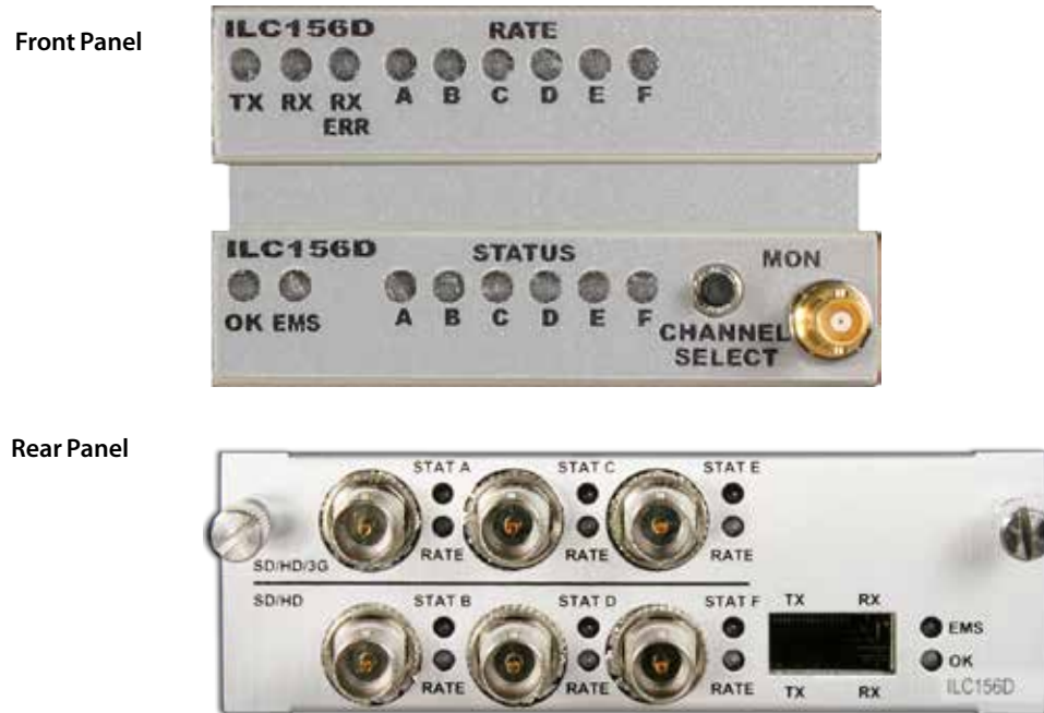
Figure 14. ILC156D Status LEDs and Monitor Connector
